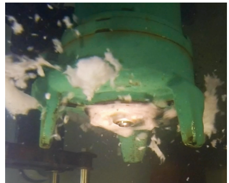
Axial cutter shredding a wipe
